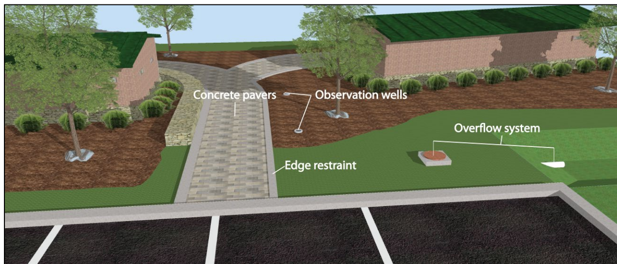
Figure 14-1. Typical NCDOT PICP sidewalk installation at a Rest Area
