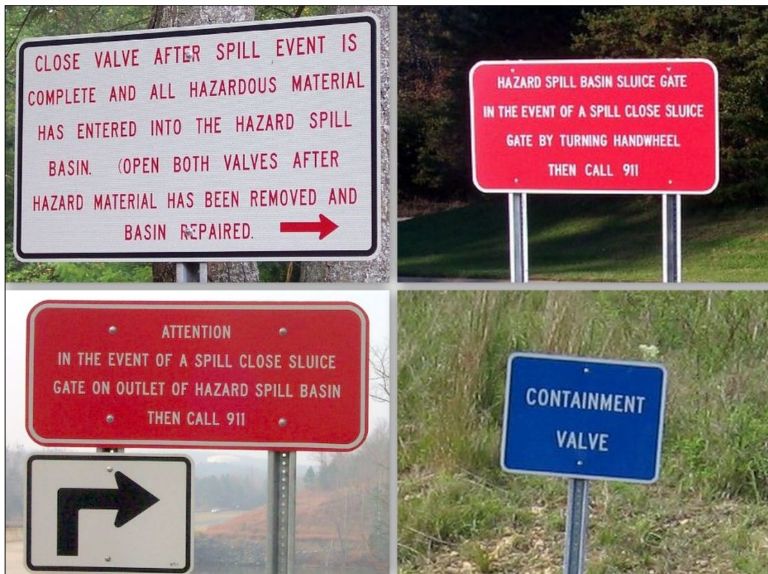
Figure 10-11. Signage associated with HSBs
